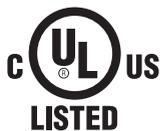
The system fulfils the Canadian and U.S. safety requirements (UL LISTED, in accordance with UL 61010A-1:02 and CAN/CSA-C22.2 No. 61010-1-04).
