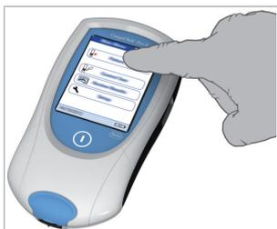
You can open any displayed function by touching (or tapping) the button for it with your finger (or a special pen for this purpose). “Tap” means: Touch the button, then remove your finger from the touchscreen. The next screen appears once you remove your finger.
