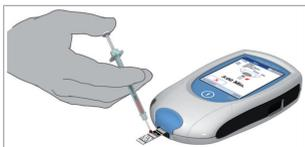
If too much blood has been applied ( $> 20 \mu\text{L}$ ) the exterior of the meter and the test strip guide should be cleaned and disinfected.
